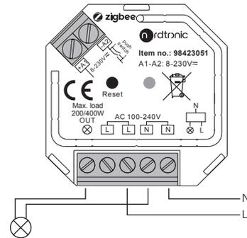
**Step 3:** power on the device, it will be set into network pairing mode (connected light flashes twice slowly), the network pairing mode will last until the device is added to a Zigbee network.
