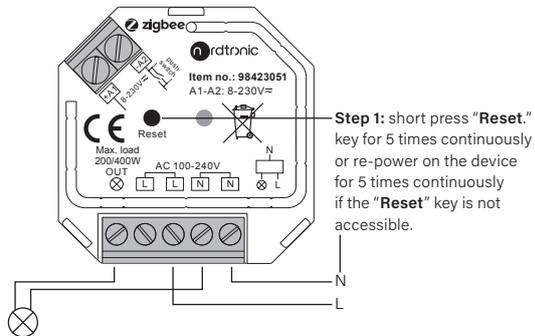
**Step 2:** Connected light will blink 3 times to indicate successful reset.
